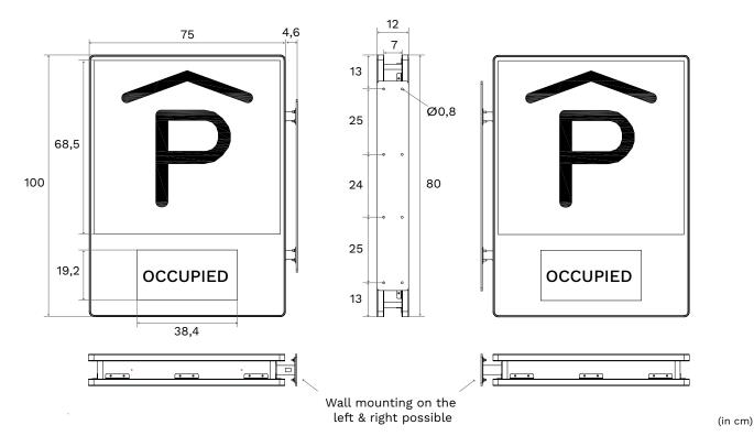
Dimensions of the free/occupied sign (for wall mounting on the rear)
